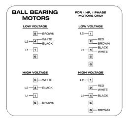
**NOTE:** Single phase motors are protected with inherent overheating devices and do not require external overload protection.
